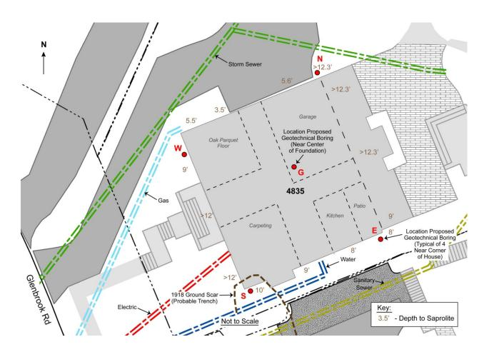
Figure 2-3 Geotechnical Boring Locations Map
